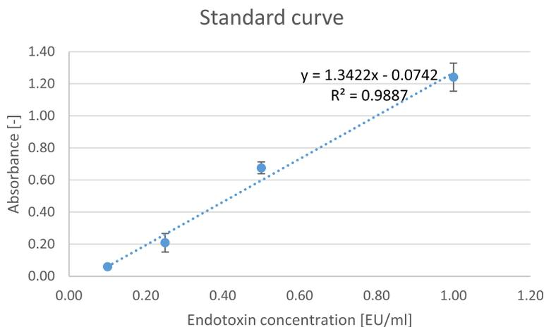
**Fig. 2** Endotoxins concentration standard curve using using Pierce Chromogenic Endotoxin Quant K, prepared according to the manufacturer's instruction.  $R^2 = 0.9887$
