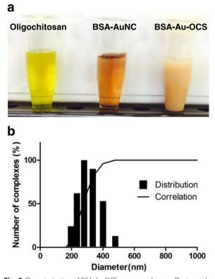
**Fig. 2** Characterization of BSA-Au-OCS nanocomplexes. **a** Photographs of BSA-Au NCs and BSA-Au-OCS nanocomplexes. **b** Size and size distribution of BSA-Au-OCS nanocomplexes
