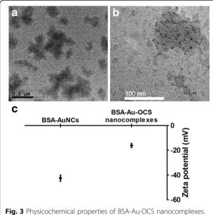
**Fig. 3** Physicochemical properties of BSA-Au-OCS nanocomplexes. Representative TEM micrographs of BSA-Au NCs (**a**) and BSA-Au-OCS nanocomplexes (**b**). **c** Zeta Zeta potential of BSA-Au NCs and BSA-Au-OCS nanocomplexes. Values are mean $\pm$ SD (n=4)
