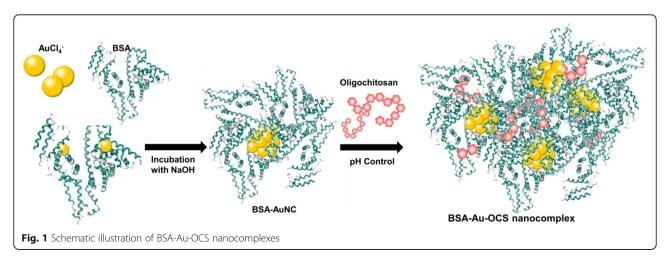
mechanical stirring. Acetic acid solution (900  $\mu$ L, 1%) was added dropwise to the mixture to reduce pH to 6.0 and the reaction was allowed at room temperature for 6 h. The prepared BSA-Au-OCS nanocomplexes were obtained by centrifugation at 9000×g for 10 min and dispersed with 1 mL of distilled water. Solid BSA-Au-OCS nanocomplexes were obtained by freeze drying and stored at 4 °C before use.
