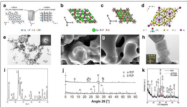
**Fig. 2** Schematic illustration of the crystal structure of (a) HAP [172], (b)  $\alpha$ -TCP, (c)  $\beta$ -TCP [173], and (d) WH [114]. Copyright 2013 American Chemical Society. TEM and SEM images of (e) HAP [174], (f)  $\alpha$ -TCP, (g)  $\beta$ -TCP [175], and (h) WH [117]. XRD data of (i) HAP [174], (j)  $\alpha$ -TCP and  $\beta$ -TCP [175], and (k) WH [117]
