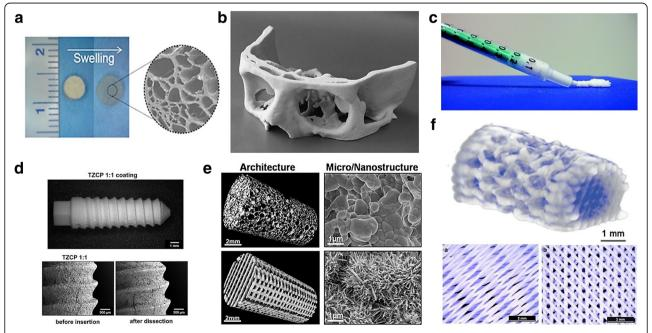
**Fig. 3** Calcium phosphate based applications. (a) WH incorporated hydrogel scaffold [116, 176]. (b) Cranial segment made of tetracalcium phosphate and β-TCP [177]. (c) The injectable paste included calcium phosphate nanoparticles [178]. (d) Mixed zirconia calcium phosphate deposited on dental implant [179]. (e) 3D printed calcium-deficient HAP scaffolds [180]. (f) 3D printed calcium phosphate cement [181]
