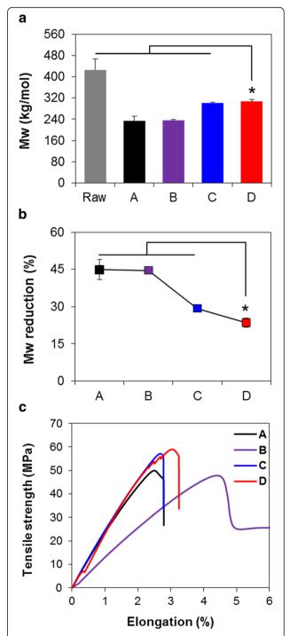
**Fig. 6** Effects of the additives on PLLA based composite films on **a**, **b** molecular weight and **c** tensile properties: A) processed PLLA, B) PLLA90/PLCL10, C) PLLA100/Mg5, and D) PLLA90/PLCL10/Mg5 blends ( $^*p$  < 0.05)
