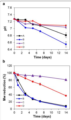
**Fig. 7** Degradation study of **a** changes of pH and **b** reduction of molecular weight with hydrolytic time: A) processed PLLA, B) PLLA90/PLCL10, C) PLLA100/Mq5, and D) PLLA90/PLCL10/Mq5 blends
