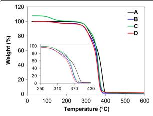
**Fig. 5** The TGA thermograms of processed PLLA and PLLA blends: **a** Raw PLLA, **b** Processed PLLA, **c** PLLA90/PLCL10 (50:50), and **d** PLLA90/PLCL10 (75:25) blends
